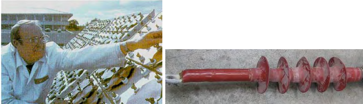
Figure 3: Long term UV Materials testing in a desert area and termination in service in a high UV environment
